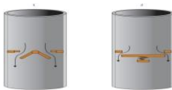
FIGURE 12: SCHEMATIC REPRESENTATION OF NON-RETURN VALVE (LEFT) CLAPPER TYPE AND (RIGHT) SPRING TYPE
